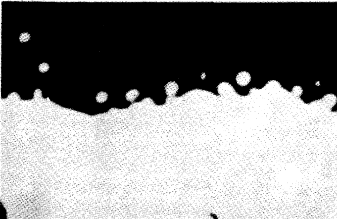
FIG. 2. Formation of domains near a moving domain wall in an ultrahigh field.
