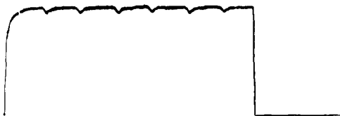
FIG. 1. Oscillogram of microwave pulse passing through the resonator: \tau_p = 1.8 msec, T = 1.2 K, H = 2.1 kOe, P/P_c = 14 dB.
