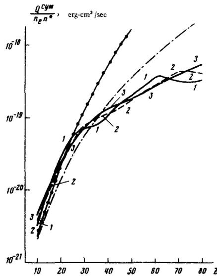
FIG. 3. Dependence of  $Q^{\text{sum}}$  on  $Z$ : 1)  $T_e = 10$  keV, 2)  $T_e = 20$  keV, 3)  $T_e = 40$  keV; dash-dot line—two-term formula of<sup>[13]</sup>, line with points—three term formula of<sup>[2]</sup>, both for  $T_e = 10$  keV.
