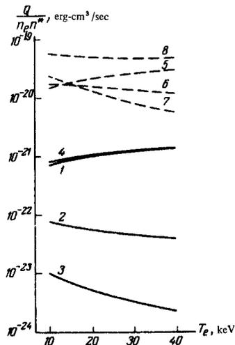
FIG. 1. Plots of  $Q^{br}$  (curves 1 and 5)  $Q^{rec}$  (2 and 6),  $Q^{lin}$  (3 and 7), and  $Q^{sum}$  (4 and 8) for carbon (solid curves 1-4) and iron (dashed curves 5 and 8) as functions of  $T_e$ .
