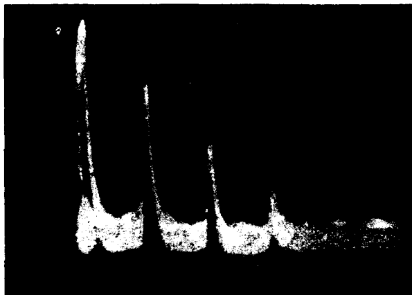
FIG. 1. Proton echo from aqueous solution of aluminate following a periodic repetition of a series of double RF pulses; \tau = 440 \mu\text{sec} ; T = 0.05 \text{ sec} . The peaks from left to right represent the response of the receiver to the second pulse and the principal, second, and third echoes.
