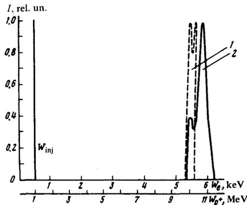
Theoretical (1) and experimental (2) energy spectra of particles accelerated with a backward spatial harmonic of a traveling electromagnetic field.
