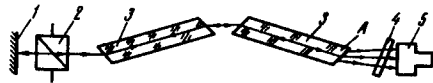
Fig. 1. Diagram of setup for obtaining and recording giant superluminescence pulses. 1 - Dense mirror, 2 - Kerr shutter, 3 - neodymium-glass rods, 4 - filter, 5 - coaxial photocell.
