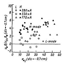
Data from JFT-2M [9]. Poloidal ion Mach number M as a function of normalized ion collisionality. Open symbols stand for the L mode and closed symbols for the H-mode
