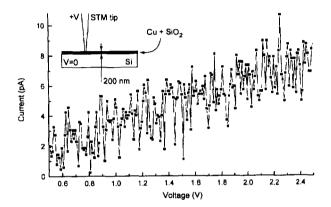
Fig.1. IV curve taken with STM tip pressed into surface across the film. T = 300 K. The squares are data points of single scan from left to right. The fine line is a guide for the eye
