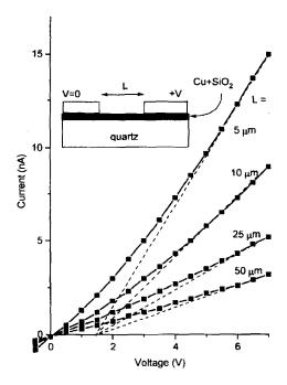
Fig. 2. IV curves taken along the film. T=300 K. The probes are 400  $\mu m$  wide and separated by a gap of L ( $\mu m$ ). The solid lines are guides for the eye. The dashed lines give the linear asymptotes with the same offset of 1.76 V. At voltages  $7 \le V \le 20$  V all the curves are straight lines (not shown) coinciding with the indicated asymptotes
